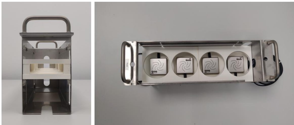
Figure 10: A custom holder designed to retrofit a Chemspeed Swing (XL) system with four magnetic stirrers.
