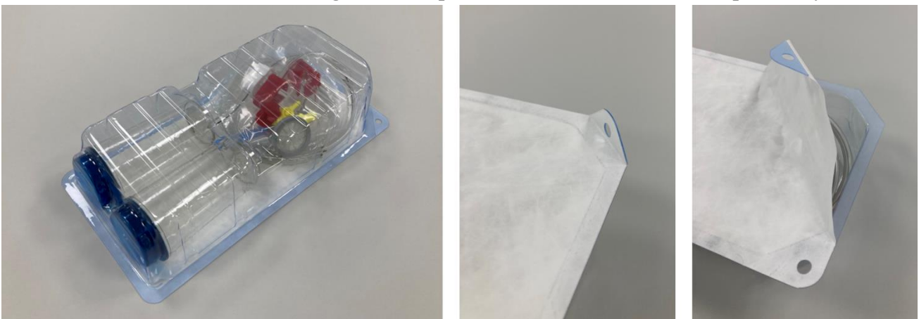
Figure 7: The sterility testing kit used by TraceBot.
