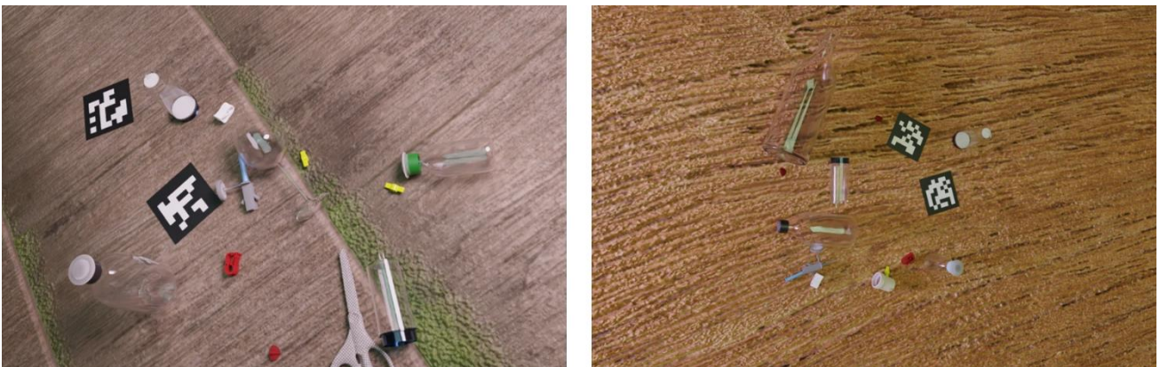
Figure 4: Two synthetic images from the dataset that was used to train TraceBot's pose estimation network. Artificial backgrounds were used to make the network more robust
