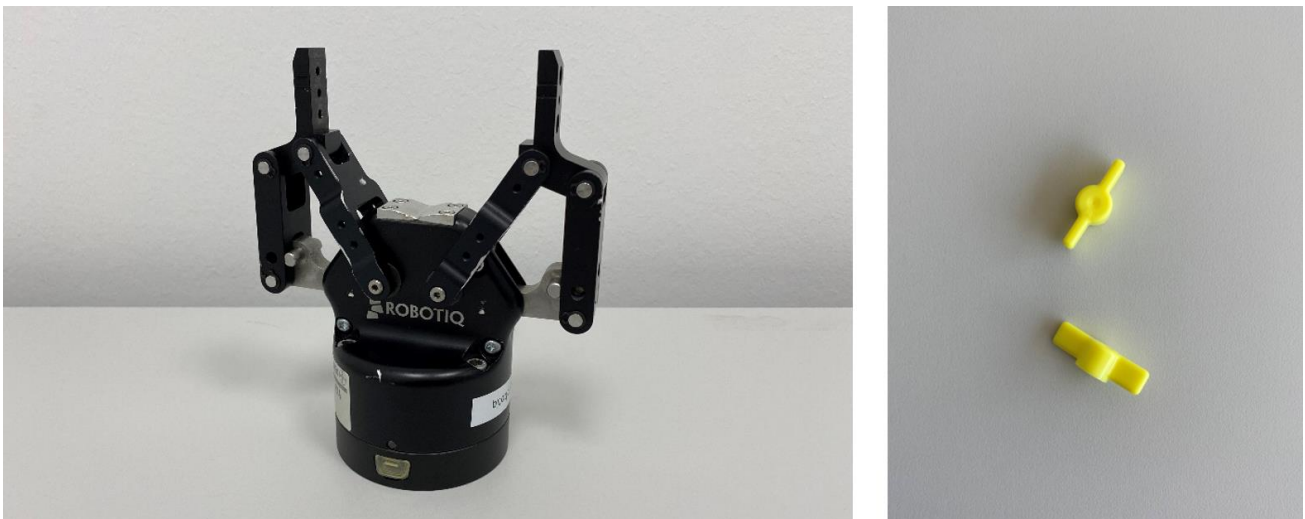
Figure 1: A parallel gripper (left) and the two yellow caps that need to be attached to the bottom of the canisters of the sterility testing kit used by TraceBot (right).
