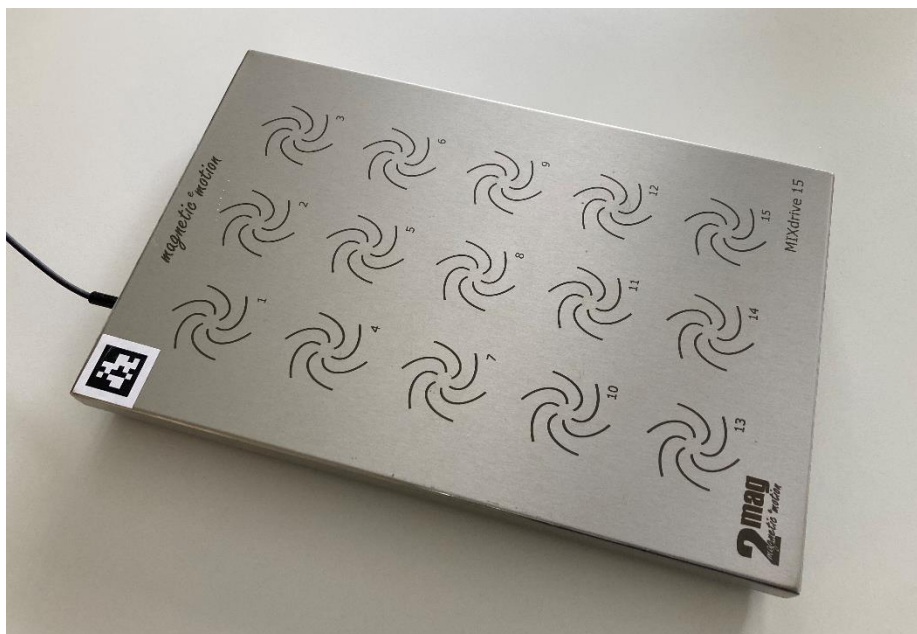
Figure 2: A magnetic stirrer with 15 stirring points.
