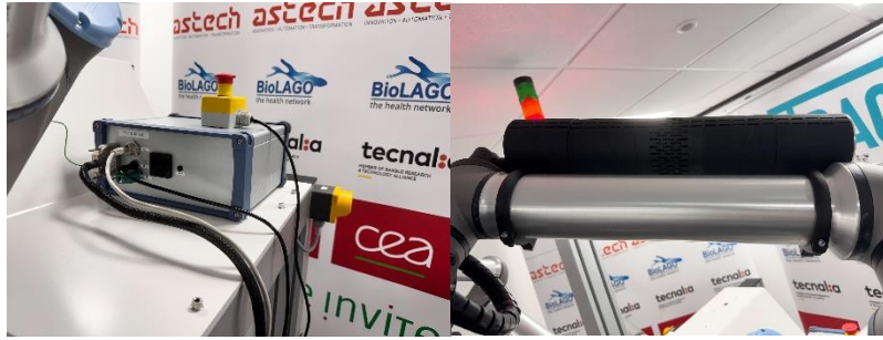
Figure 3: External controller unit and the motor driver of the CEA Gripper
